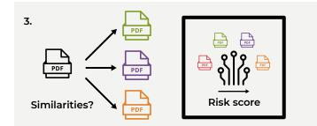
If the hash can't be located in any database, the local engine calculates a risk score based on ML algorithms. Only if the risk level exceeds a certain threshold, the file is uploaded to the cloud.
